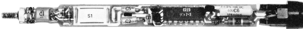
PART NO. 00546-60001 CIRCUIT BOARD SERIES 1608, 1616, AND 1624. (BREAKDOWN DIODE CR1 ONLY IN SERIES 1624)
